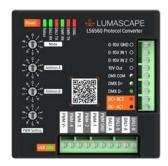
Lumascape's LS6560 Protocol Converter has been designed to convert DMX to PWM, DALI to PWM, DALI to DMX and 0-10V to PWM. This effectively allows for seamless integration of Lumascape products into most commercial lighting installations.
