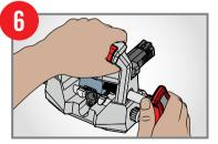
Turn Easy Torque Handle™ and push sight through dovetail slot.
