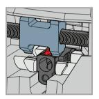
Use this step to ensure everything has remained aligned during the locking process and that the press block remains in correct alignment with the sight or dovetail slot and completely clears the slide to prevent damage.
