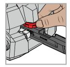
Once the upper frame is moved to the correct position, lower the Vertical stabilizer to the top surface of the slide to completely lock into place prior to pushing sight.
