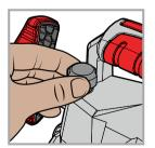
Turn both frame bolts simultaneously to avoid binding and keep upper frame level
