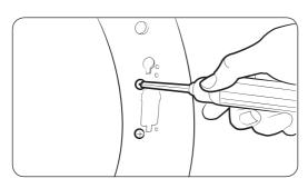
**5.** Remove the two screws that are above and below the cut-out in the frame front.
