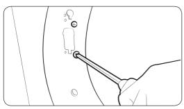
**8.** Re-insert the two screws that held the lever holder into the same screw holes, and then tighten.
