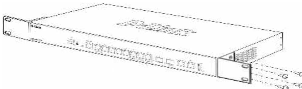
Figure 2 — Attaching rack-mount brackets to the Switch
