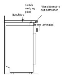
INSTALLING THE MACHINE 9
