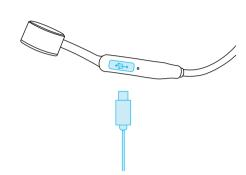
Plug in the included charging cable. The LED will be red when charging and turn blue when fully charged.
