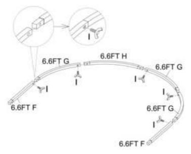
Step 2: Assemble Part B as shown using hardware I.
