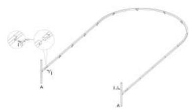
Step 4: Assemble Part "8FT C", "8FT D" & "8FT E" as shown using hardware I. Then use part J to install them onto the frame you completed in the previous step. The position of the assembled part I on the component before locking part J can be adjusted according to your needs.
