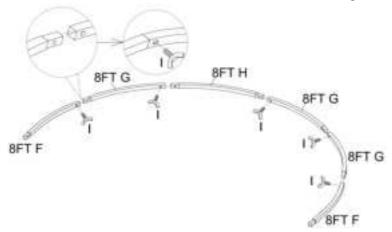
Step 2: Assemble Part B as shown using hardware I.
