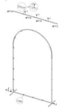
7.2ft Step 1: Assemble Part "7.2FT F" , "7.2FT G" & "7.2FT L" as shown using hardware I.
