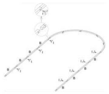
Step 3: Assemble Part A as shown using hardware I.
