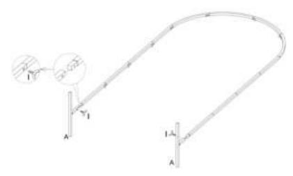
Step 4: Assemble Part "6.6FT C", "6.6FT D" & "6.6FT E" as shown using hardware I. Then use part J to install them onto the frame you completed in the previous step. The position of the assembled part I on the component before locking part J can be adjusted according to your needs.
