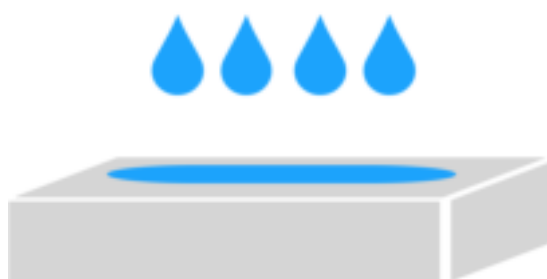
Figure 5: Liquid odorant dispensed onto the sponge material.
