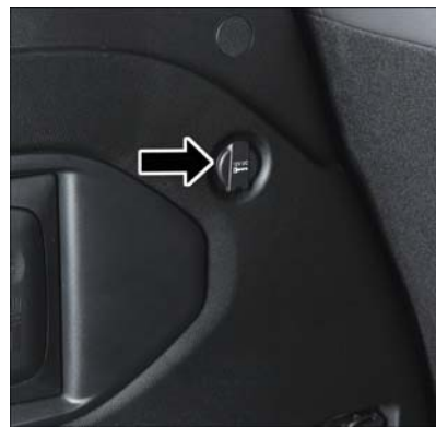
Rear Cargo Power Outlet
