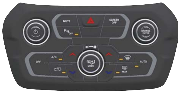
Automatic Temperature Controls (ATC)
