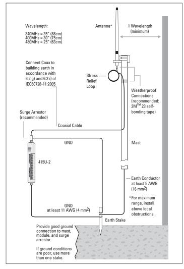
Figure 9. Antennas installation - Collinear/Dipole
