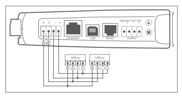
Figure 12. RS-485 connections
