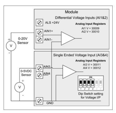
Figure 22. Single-ended voltage inputs
