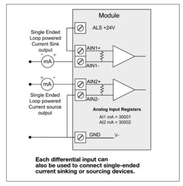
Figure 20. Al1 and Al2 single-ended current inputs
