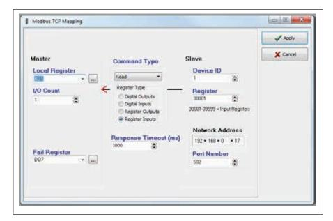
Figure 62. Modbus TCP client mapping
