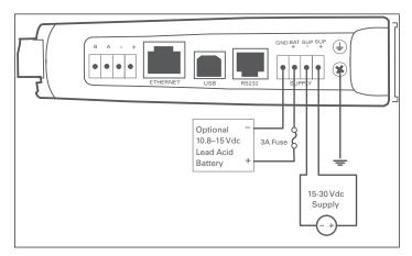
Figure 6 Supply connections
