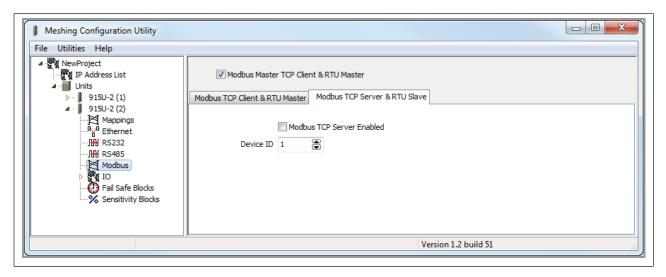
Figure 60. Modbus TCP server and RTU slave tab
