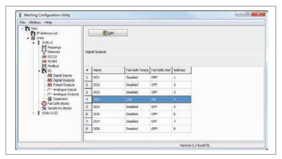
Figure 17. Digital output fail-safe times
