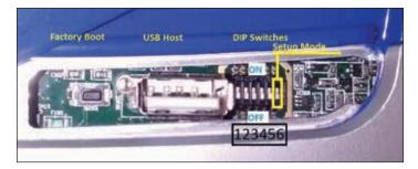
Figure 101. Module USB port and switches
