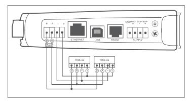
Figure 7. Expansion I/O power and RS-485
