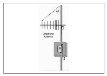
Figure 9. Directional antenna
