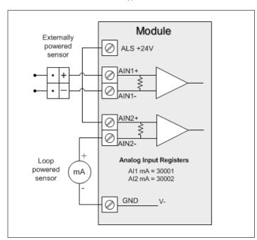
Figure 19. Differential current inputs (Al1 and Al2)
