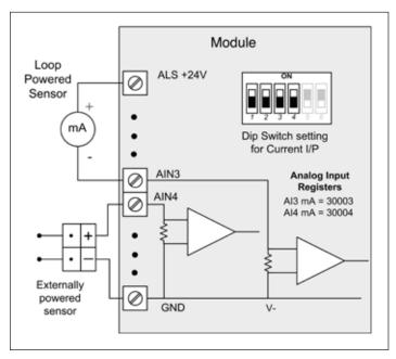
Figure 21. Al3 and Al4 Single-ended current inputs
