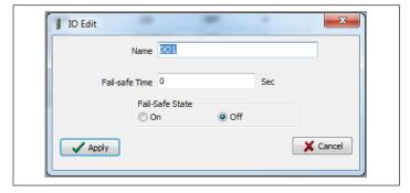
Figure 41. IO edit (digital output
