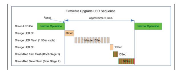
Figure 102. Firmware upgrade LED indicators
