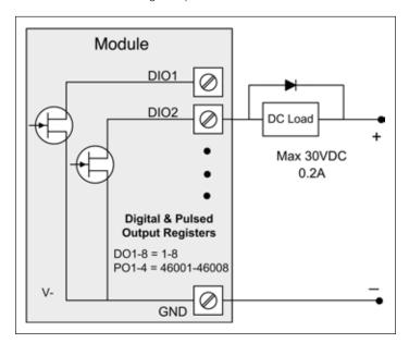
Figure 16. Digital pulsed output wiring
