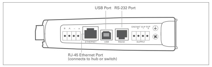
Figure 11. Bottom panel connections
