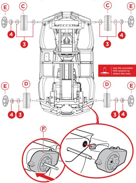
Put the rear wheel, gasket and nut into the rear axle in turn. Fix the nut with a wrench, and then fix the wheel cover on the wheel.
