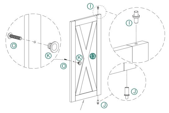
Large hole to install J, small hole to install I
