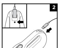
2. Plug the USB-C end of the charging cord into the port on the handle. Plug the USB end of the charging cord into a compatible USB outlet cube or adaptor (not included) and plug into a wall outlet.
