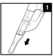
**1.** To remove an accessory, slide it straight off the nozzle.
