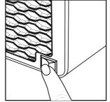
2. Power on the main unit using the switch at the back of the unit.
