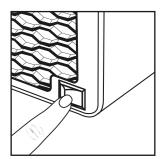
7. Turn off switch at the back of unit to shut the unit off completely.
