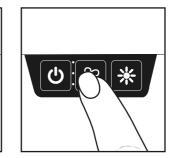
4. To adjust fan speed, press to choose HIGH, MEDIUM, or LOW. High - 3 lights on Medium - 2 lights on Low - 1 light on
