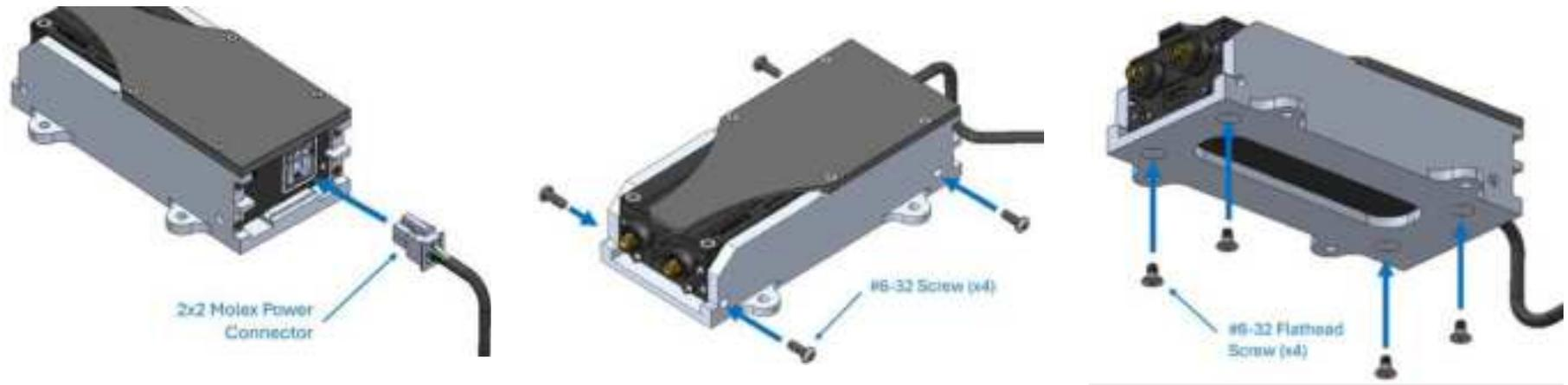
**Connections:** Insert power cable, 2x2 Molex (shown with guide marker toward the top of the device), per ICD specifications.
