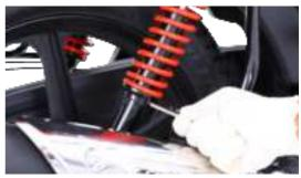
If the spring is adjusted to maximum notch, then it will be stiffer which is good for heavy loads.
