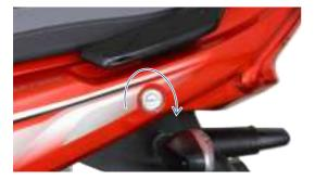
Seat lock is provided at the tail end of the vehicle for the removal of seat assembly and there by accessing the tool kit and first aid kit. Follow the procedure given below for removing and re-fixing the seat assembly.
