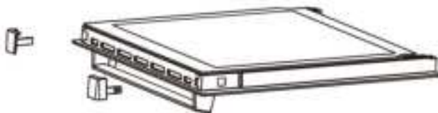
Removal of the internal glass panel
