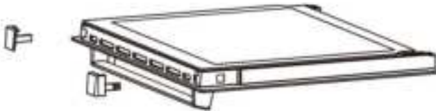
Removal of the internal glass panel
