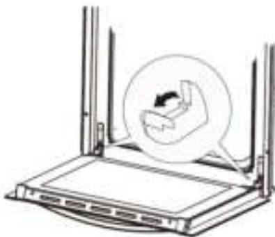
Tilting the hinge safety catches
