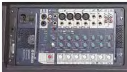
STAGEPAS-500 SHOWING 10-CHANNEL POWERED MIXER
