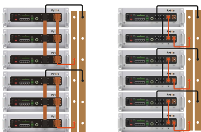
Figure 5-1 Schematic diagram of power cable connection
