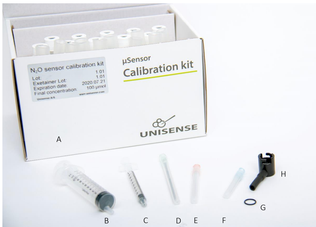
Figure 1: Calibration kit contents: A: Calibration kit box with Exetainers and ampoules, B: 10 ml syringe, C: 1 ml syringe, D: 80 x 2.1 mm needle (green), E: 50 x 1.2 mm needle (red), F: 30 x 0.6 mm needle (blue), G: O-ring, H: Calibration Cap with tubing.
