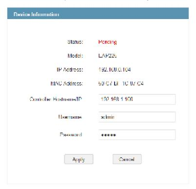
7. Click **Apply** to inform the EAP of the OC200's hostname or IP address. Then the connection can be established between the EAP and the OC200.
