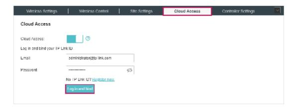
The TP-Link ID which is bound with the OC200 for the first time will be automatically bound as an administrator. And only one TP-Link ID can be bound with the OC200 as an administrator. An administrator account can add or remove other TP-Link IDs to or from the same OC200 as Cloud Users.
