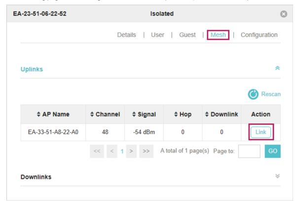
Once adoption has finished, your device can be managed by the OC200 in the same way as a wired EAP. You can click the EAP's name on the Access Points tab to view and configure the mesh parameters of the EAP on the pop-up window. Please refer to View Mesh Information of the EAP.
