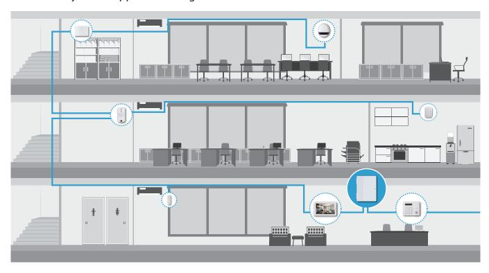
Hybrid Panel Lite simplifies installation and improves flexibility by utilizing BUS connectivity, allowing shorter wiring lengths which makes it easy for users to expand the system by connecting multiple devices to a single BUS line.
