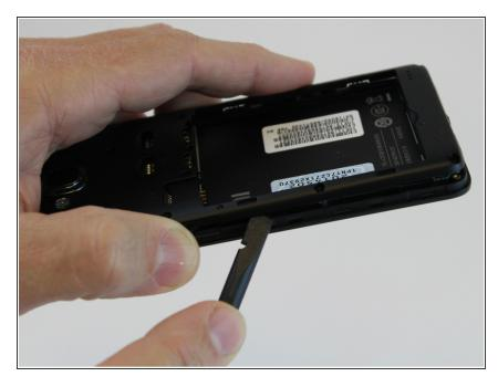
Slide the spudger between the midframe and front body, gradually prying the two bodies apart as you slide the spudger around the perimeter of the phone.
