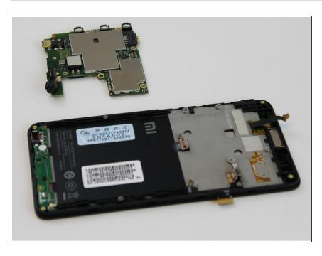
Lift the motherboard out of the front cover and set aside.
