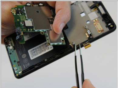
• Using the tweezers, pull the antenna connector from the motherboard.
