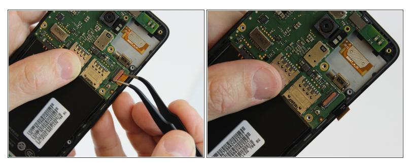
Using one prong of the tweezers, pry back the brown clip located on top of the LCD ribbon connector.
