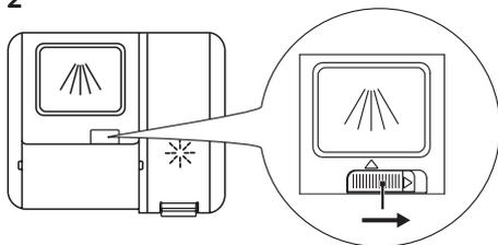
Slide the release catch to right, then open the cap of the detergent dispenser
