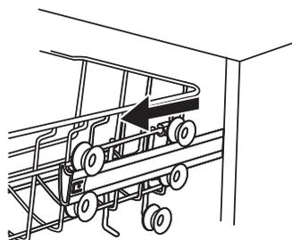
2. Re-attach the upper basket onto the upper or lower rollers.
