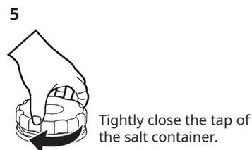
**⚠ Caution!** Water and salt may come out of the salt container when you fill it. After you fill the salt container, immediately start a programme to prevent corrosion.
