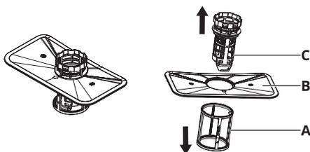
3. Rinse the filters (A), (B) and (C) with water. If necessary, use a soft cleaning brush.
