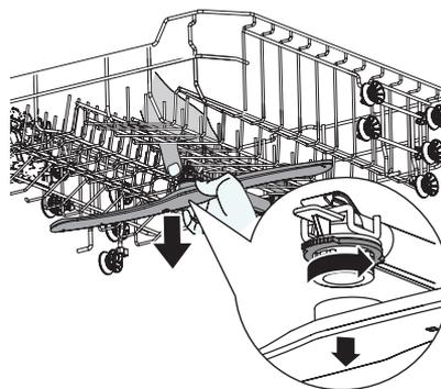
3. To detach the lower spray arm from the bottom of the appliance, just pull it up to remove.
