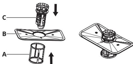
5. Insert the filter assembly into position, and turn it clockwise until it locks. Make sure the arrows on the filter (B) and (C) are aligned, as shown in the figure below.
