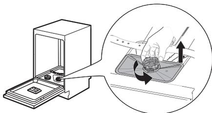
2. First pull the filter (A) out of the filter assembly by compressing it gently. Then the filters (B) and (C) can be detached.
