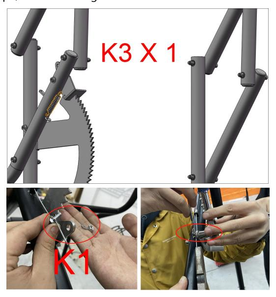
Note: Clamp the wire rope with a pliers and string in the screw, screw in the screw, clamp the wire rope and adjust the screw to the proper position
