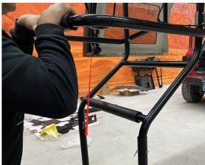
4. We recommend that the two support devices in front of you support the two large boards in front of the hardtop, and the four support devices in the back support the edge of a small board on one side. As the picture shown.
