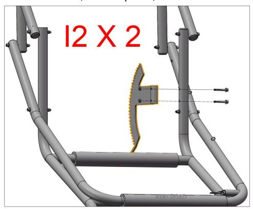
2 Install the adjustable travel stop (Part "K1" in screw pack 4) in the second hole on the side with the handbrake.
