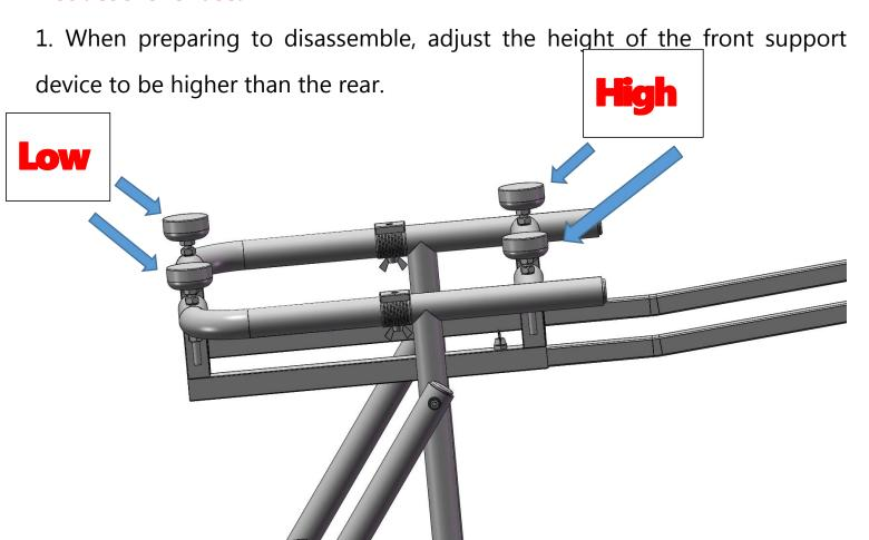
2. After the roof is stuck, install the front supports (Part "F")The front of the first roof should be significantly higher than the rear, and the recommended distance is about 4 inches, as shown in the figure below. At this time, the roof has a certain height so that it will not bump the vehicle body.
