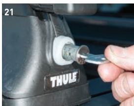
21) The button to release the foot from the base can be replaced with an optional keyed lock. 22) The Thule Big Mouth Upright Carrier mounts to the crossbars with specially designed clamps, and the wheel straps (23) slide into the wheel tray. The system does a good job stabilizing bikes for transport.
