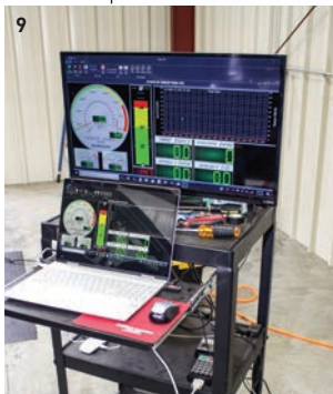
8) The 5-Star programming device plugs in to the vehicle's OBD-II port and can be left connected so it acts as a customizable digital-gauge readout. 9) The dynamometer control station shows all the vehicle data in real time and records the numbers for later analysis. The computer will immediately create charts showing vehicle performance. 10) A 5-Star Tuning technician shows the hand control for the dynamometer that he uses while running the tests from inside the truck.
