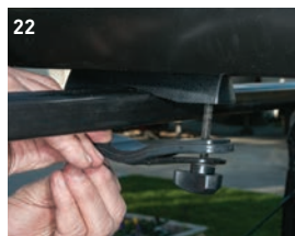
21) The button to release the foot from the base can be replaced with an optional keyed lock. 22) The Thule Big Mouth Upright Carrier mounts to the crossbars with specially designed clamps, and the wheel straps (23) slide into the wheel tray. The system does a good job stabilizing bikes for transport.
