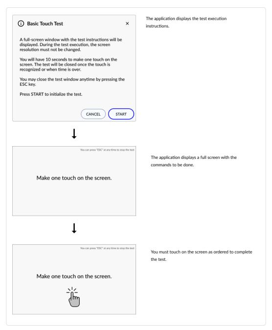
Figure 79: Basic Touch Test
