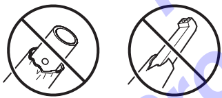
Figure 108 – Tip Sleeve Damage
