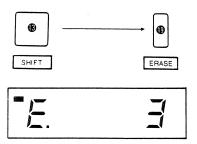
4 Press the Load Button 10, and the data is erased from the assigned measure (shown in the Display) to the end. Then the Erase mode is automatically cancelled.
