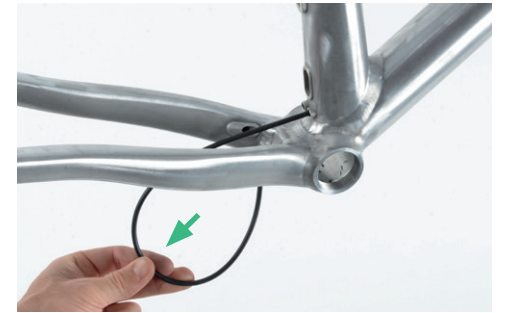
8. Twist the looping downwards in order to prevent the cable housing from breaking off.
