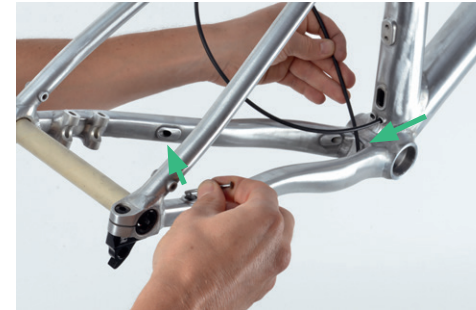
7. Push the one end of the cable housing into the chain stay until it can be seen at the rear end of the right-hand chain stay. Guide it out of the chain stay using a nail, for example, and have it exceed the chain stay with approximately 20 cm.
