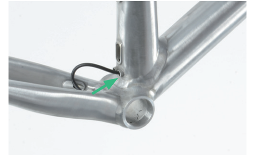
9. Push the cable housing at the steering tube and simultaneously guide the looping backwards. Make sure, the cable housing is not bent.
