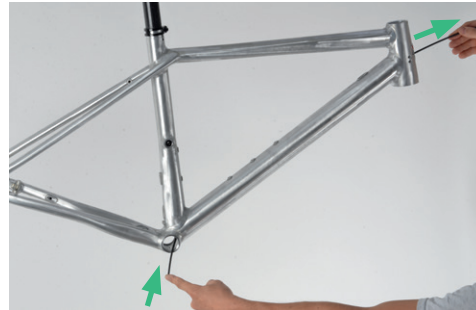
4. Pull the shifting cable housing including the foam tube back and bend the end of the cable.
