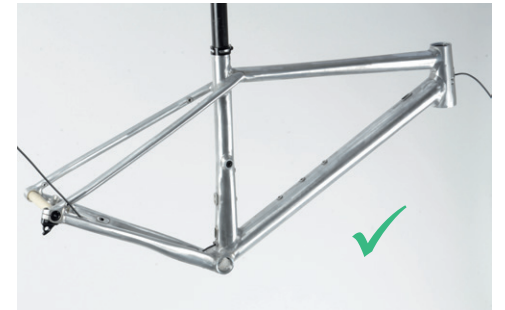
10. Cut the cable housing at both ends as needed for the final installation of the shifting components.
