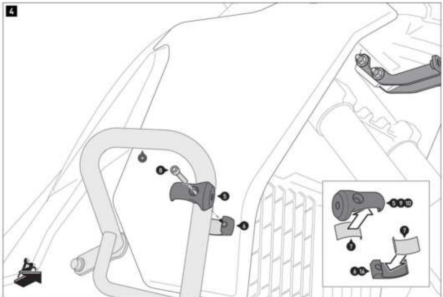
Glue the rubber strips (7) in clamps (5), (6), and (16) as well as in the clamps of the crash bars (9/10) as shown in the detailed drawing. Screw the clamps (5/6) onto the SW-MOTECH crash bar. **▲ WARNING: Use a liquid threadlocker!** Do not tighten the screws (8) yet.
