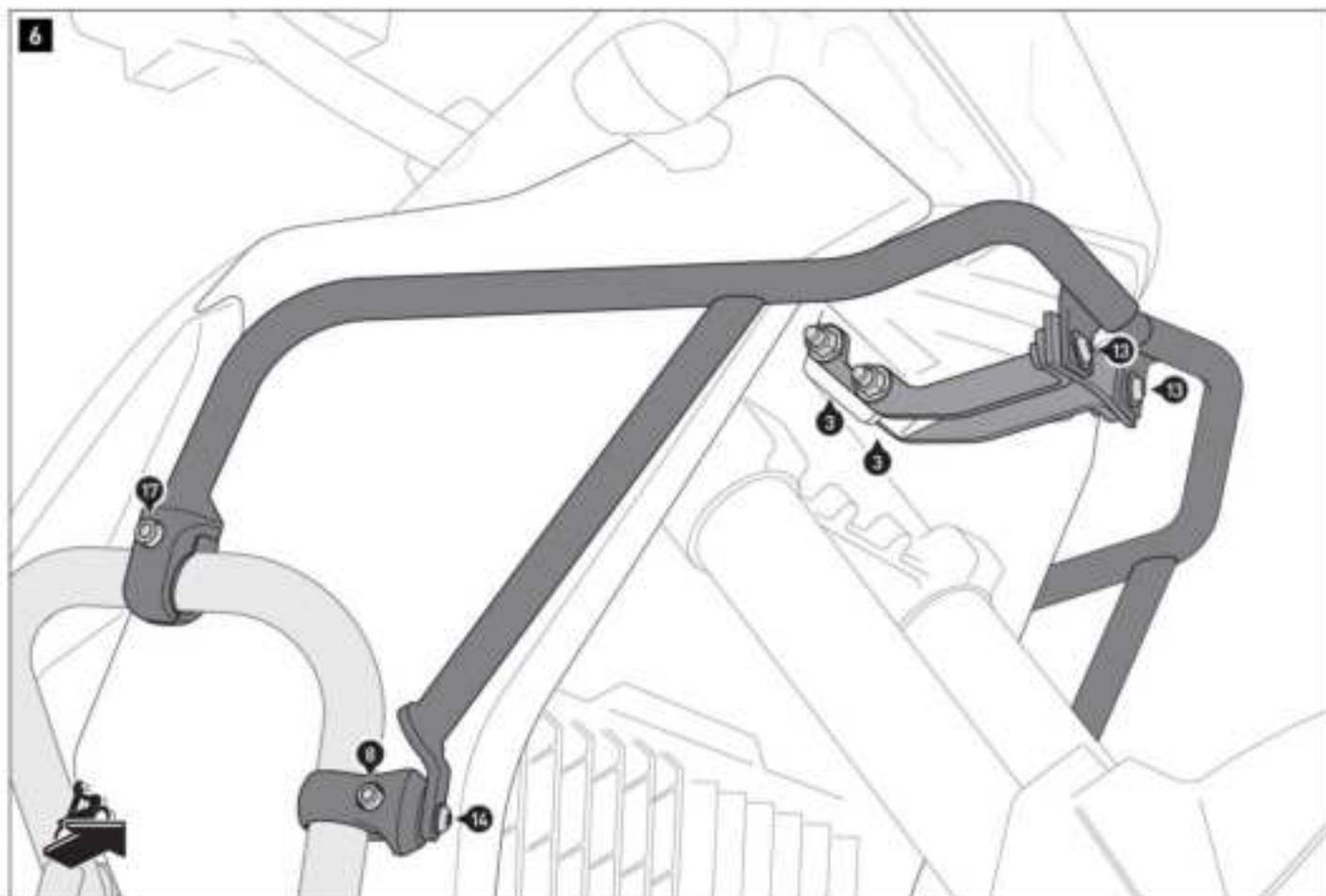
When all parts are seated without tension, tighten screws (3), (8), (13), (14) and (17) as specified in the mounting instructions.
