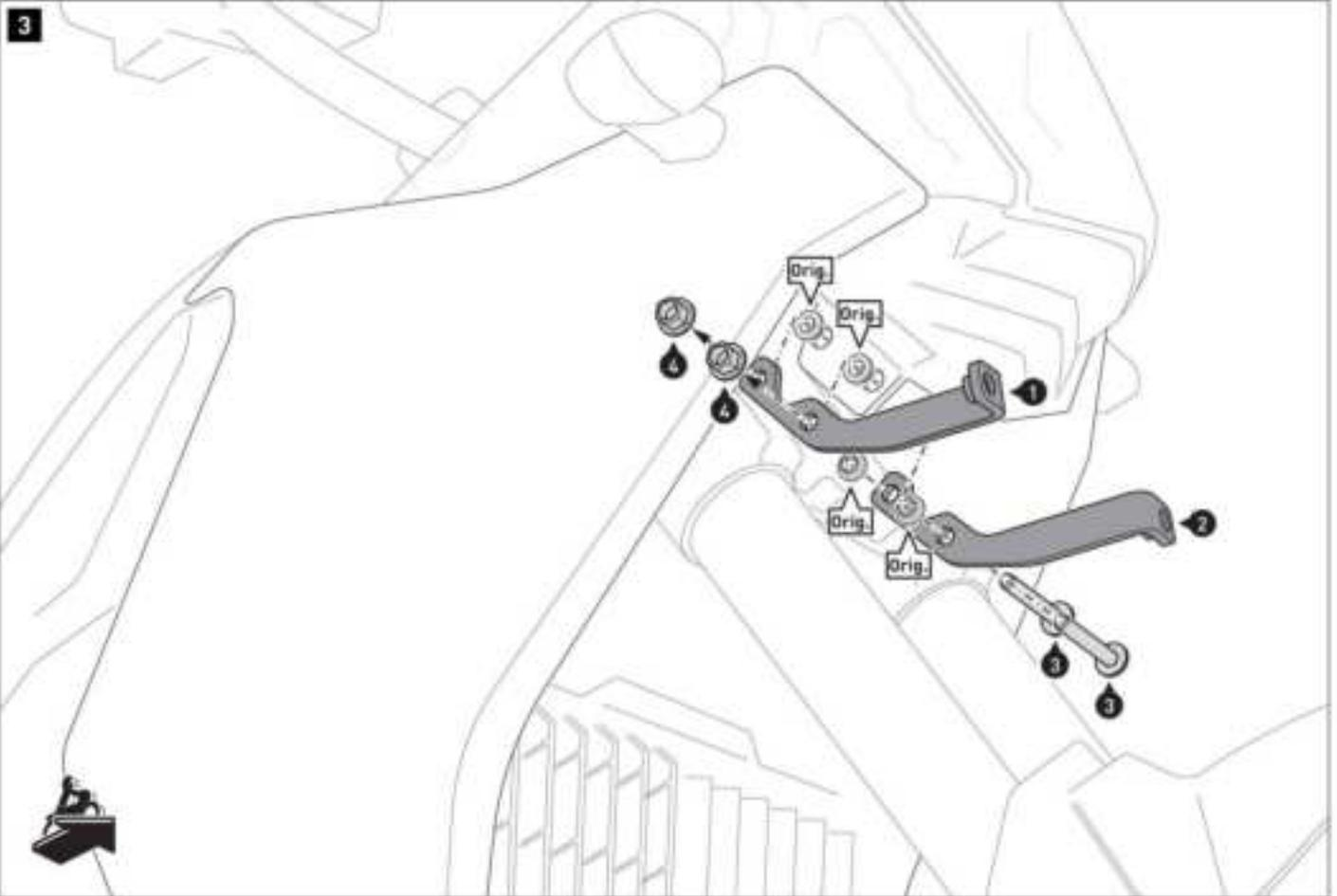
Screw the mounting brackets (1/2) onto the vehicle using the original spacers (Orig.).
