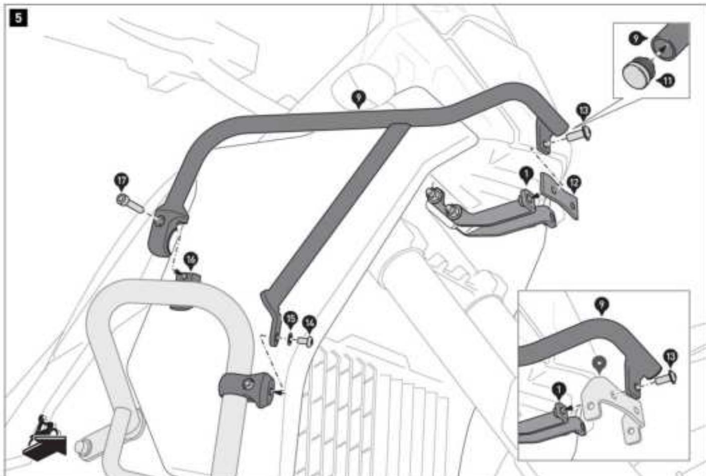
**NOTE:** When installing the crash bar with the SW-MOTECH headlight holder, use the mounting bracket (\*) of the headlight holder as shown in the detailed drawing.
