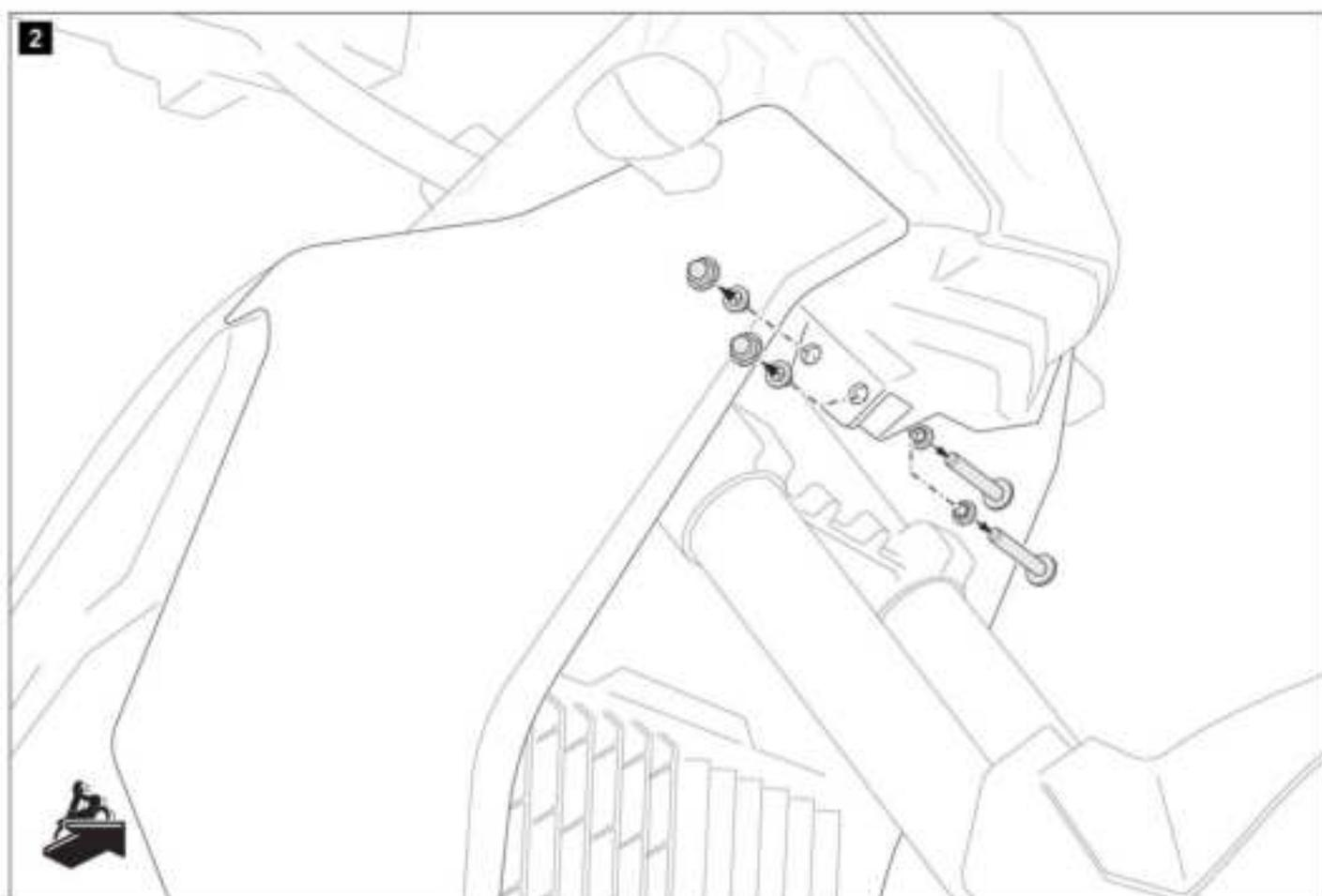
Remove the original parts from the attachment points shown.
