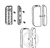
7.3 Change the battery and change the Wi-Fi network In the case of the battery is over or the Wi-Fi network is changed (Wi-Fi name or password is changed), take down the device part, to replace the battery or config the Wi-Fi network again;
