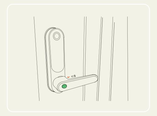
Mount both handles. The **exterior door handle** has a **hole** for the key cylinder. Place the handles in the desired direction for your door and use the supplied tool/bit to fasten the screws.
