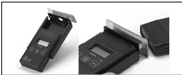
Figure 6. 718 Static Sensor charging plate in use.
