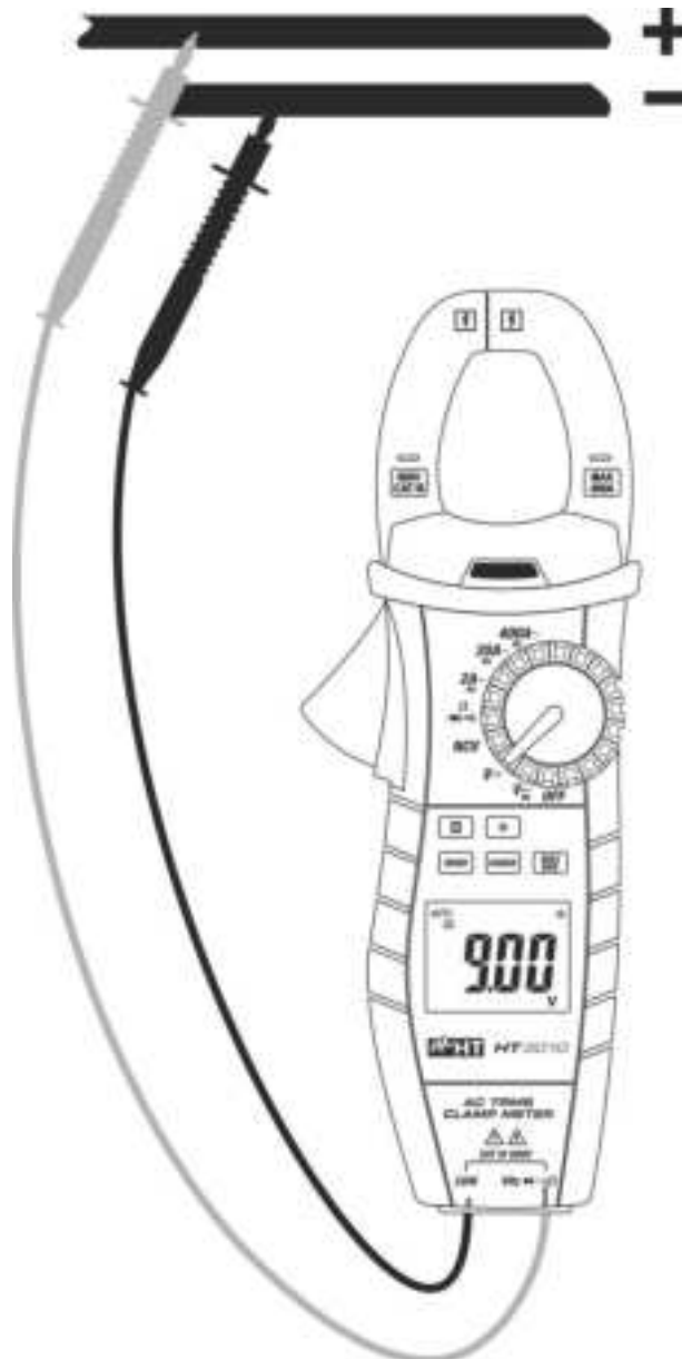
Fig. 3: Use of the instrument for DC Voltage measurement
