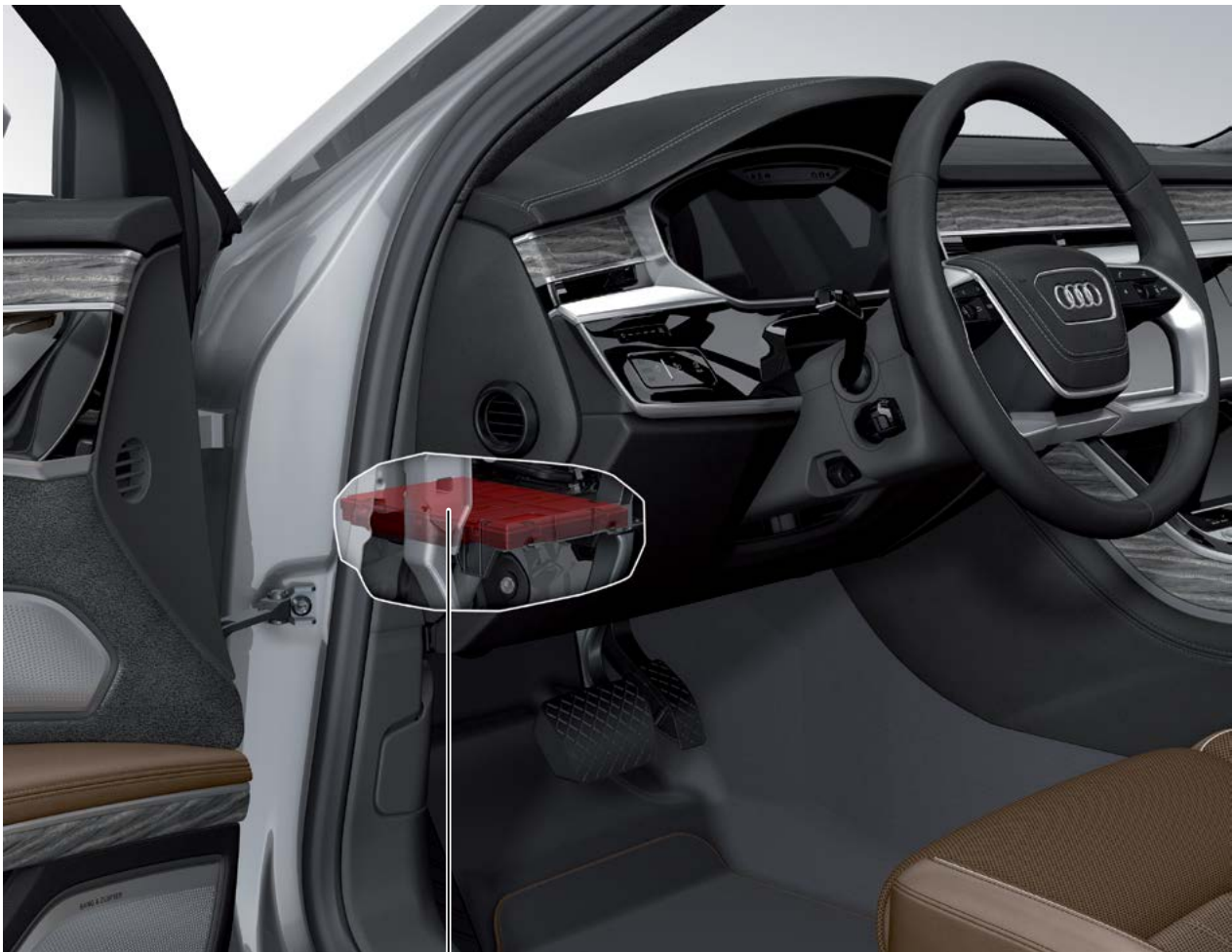
Vehicle Electrical System Control Module J519
