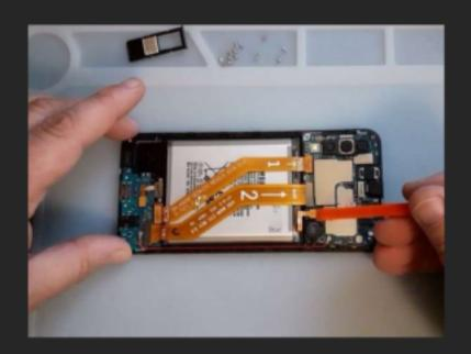
Disconnect the ribbon of the installed display and connect the new display. Connect batteries to the board and start the gadget. To play the display test: Open the Phone application, click the Keyboard option and type: \*#\*#0\*#\*#\*
