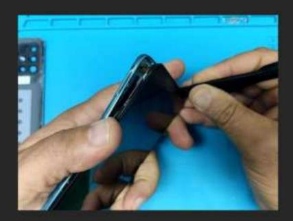
After dismantling the frame, the first thing to do is to remove the battery strap, it is necessary!
