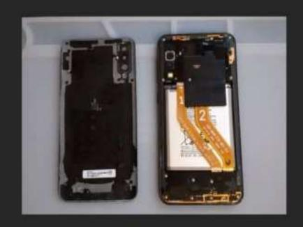
Use a screwdriver to remove all the screws from the plastic frame. Remove the plastic frame using a spatula as shown in the picture. We recommend starting to the left or right of the battery. Be aware of the tapes and cables hidden under the frame
