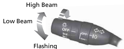
Light Control Switches
