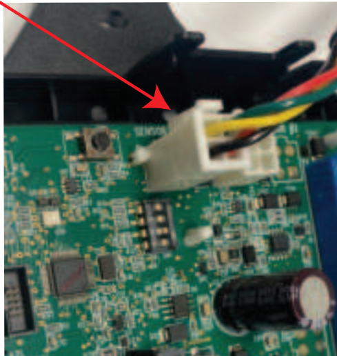
Figure 4. Connecting the RDS sensor to RDS Non-Communicating Control Board
