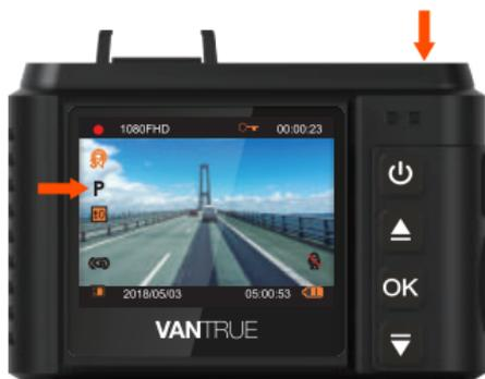
In Parking Mode, when the camera turns off, it will turn on and end recording after 20 seconds once the camera detects crash in front.
