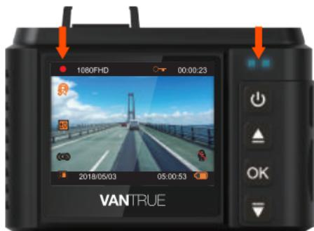
By default, the loop recording time is 3 mins. Please go to "Record Setup">"Loop Recording" to change to 1 min, 3 mins, or 5mins for your need. When it turns off, the camera will record video in 30 mins per clip, but would not overwrite the old videos when the card is full.
