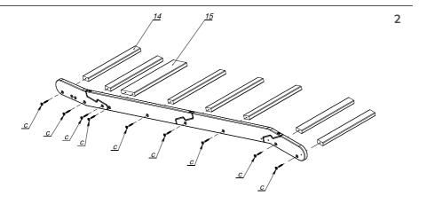
Insert beams (14, 15) into the grooves of the previously assembled side panel and screw them with self-tapping screws (c) using key (e). See Fig. 2.
