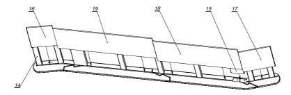
Place the previously assembled structure on the side panel so that the beams (14) are vertical. Insert panels (15-19) into the grooves. See Fig. 3.
