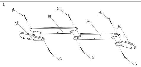
Assemble the right side panel. Sequentially connect parts 6, 8, 10, and 12 using self-tapping screws (d) and key (e). See Fig. 1.
