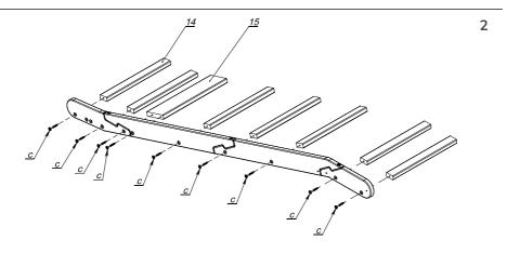
Insert beams (14, 15) into the grooves of the previously assembled side panel and screw them with self-tapping screws (c) using key (e). See Fig. 2.
