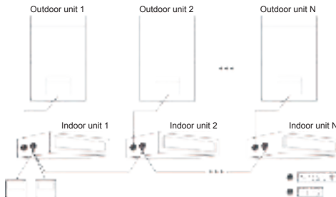
Fig. 4.9 two wired controller control multiple Atlas indoor units simultaneously
