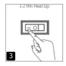
Insert the Power Plug. Press the ON/OFF button to turn the machine on, the 3 buttons start to blink blue light slowly to indicateit's heating up.
