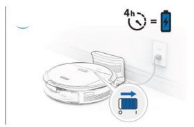
(4) Power on: Open the robot's Top Cover. Turn the robot's Power Switch to the ON position. DEEBOT is powered ON when DEEBOT emits a musical sound and the AUTO Mode Button stays illuminated.
