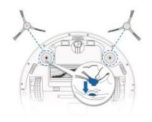
(1) Place the Charging Dock on a level floor surface and keep the immediate area 1.5m (5') in front of the charger and 0.5m (1.6') on both sides of the charger clear of objects and reflective object surfaces. Plug the Charging Dock in. (3) Install Side Brushes: attach Side Brushes to the bottom of DEEBOT by pressing a brush into each slot with the matching color until it clicks.
