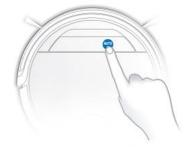
(6) Start the DEEBOT: activate the DEEBOT by directly pushing the button on its surface.
