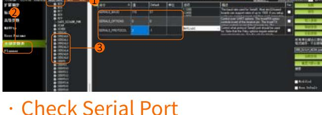
Check Serial Port Confirm that the flight controller serial port data is normal and available, and ensure that the serial port wiring is correct. Note that TX and RX must be
