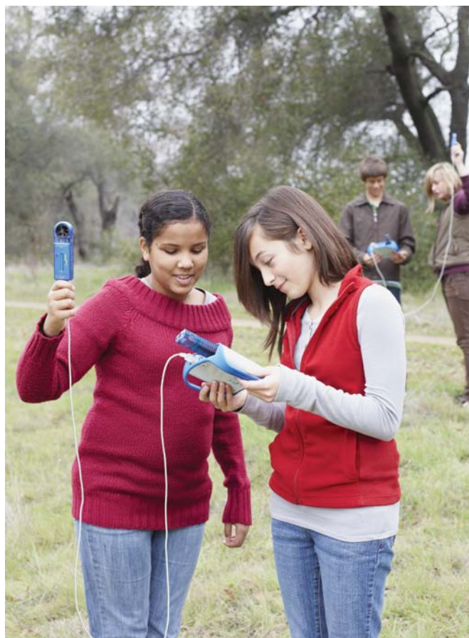
Students explore their school surroundings with the Weather/Anemometer and GPS Position Sensors – all the data is tagged with GPS coordinates for automatic mapping in My World GIS.
