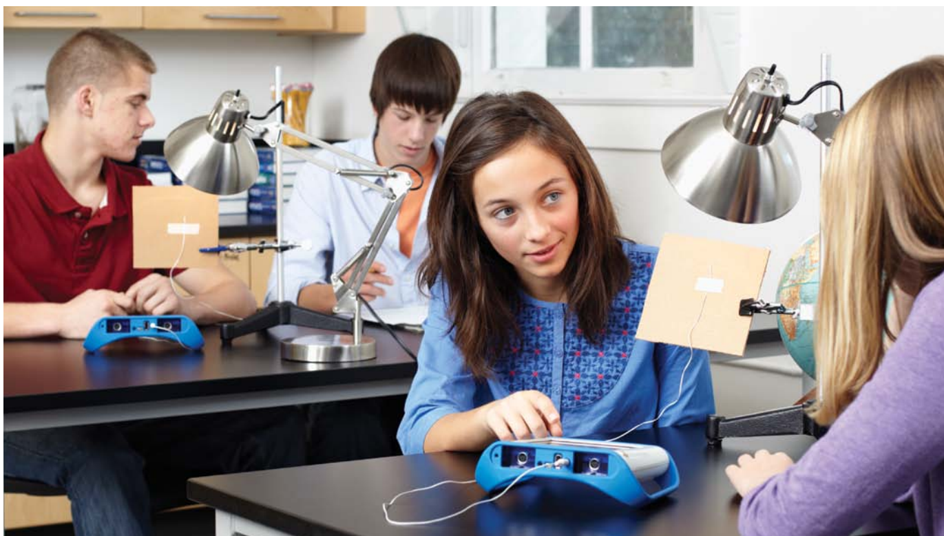
Students investigate how the angle of sunlight (using lamps) affects the temperature at the earth's surface (using cardboard), as monitored by a Fast Response Temperature Probe.
