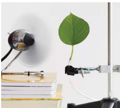
Using a fan mimics a windy environment in which a plant would experience increased transpiration.
