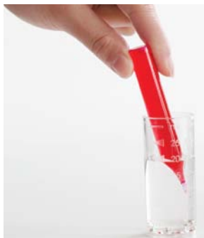
...sample instantly flows into tube, mixing with the reagent.
