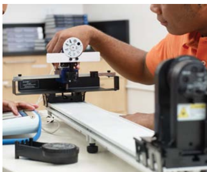
The light sensor combines with the rotary motion sensor for the diffraction of light experiment.
