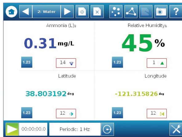
Connect your GPS Position Sensor when you're in the field and all your collected data is automatically paired to GPS coordinates.
