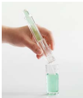
On final color change, turn titrator over and measure concentration using built-in scale. That's it!
