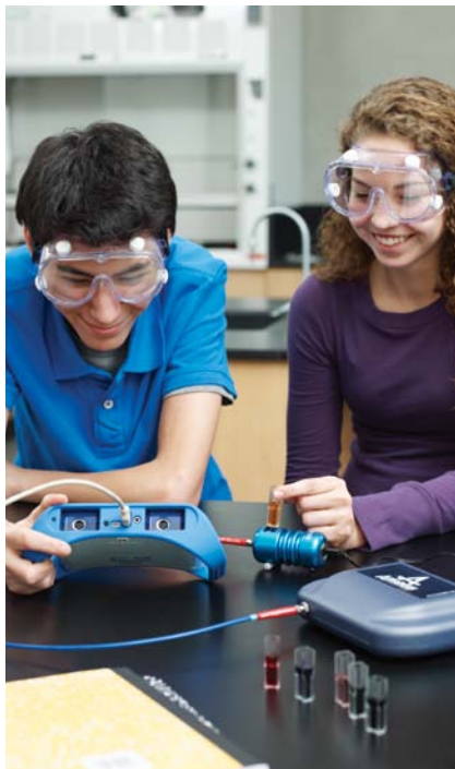
Students collect full absorption spectra to determine the concentration of species in the solution.
