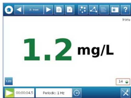
Iron concentration using ezSample Snap Vial and Water Quality Colorimeter.
