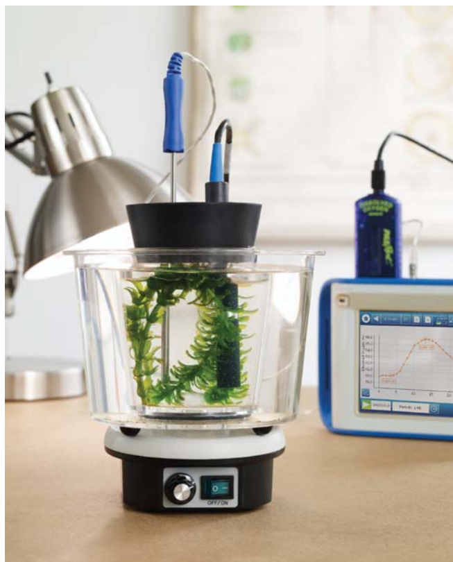
Using the Photosynthesis Tank and a Dissolved Oxygen Sensor, students measure the dissolved oxygen content in the environment of an aquatic plant.
