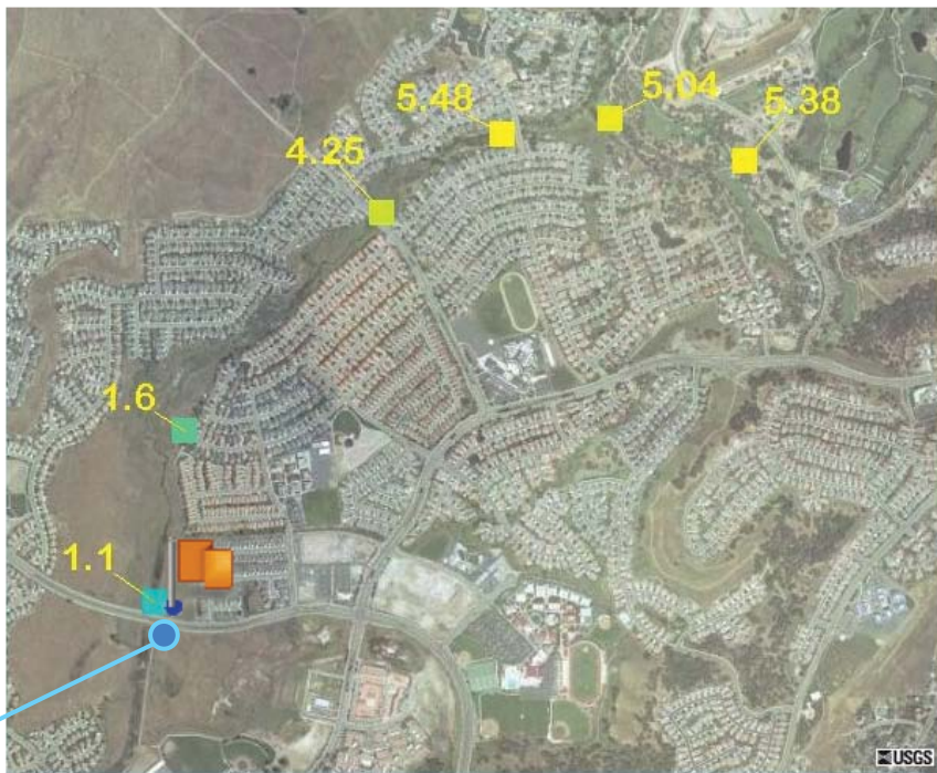
Samples of ammonia collected along a creek running from a golf course and through a development. Note the high concentrations of ammonia begin to dissipate as the creek leaves the development for open space.
