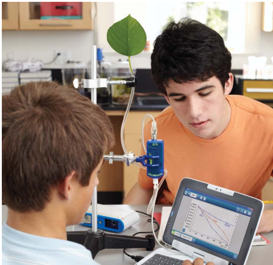
Students investigate transpiration using a very sensitive potometer that incorporates the PASPORT Barometer/Low Pressure Sensor.
