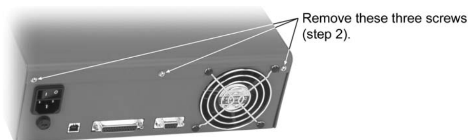
Figure 13: C7400 and C7400ER: Remove the back screws
