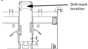
3. Remove the controller from the wall and drill four holes at the marked locations.
