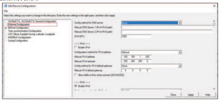
Fig. 30 Edit Device Configuration, Ethernet, and IP Settings
