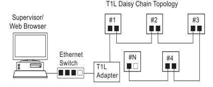
Fig. 70 IP T1L Daisy chain topology
