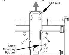
2. Hold the controller along the wall and mark drilling locations through the screw red clip slots, as shown in figure 10.
