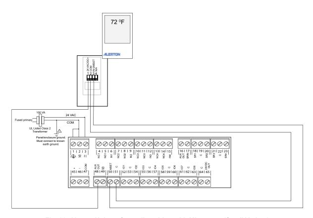
Fig. 23 Alerton Unitary Controller wiring with Microset 4 (Small Variant)
