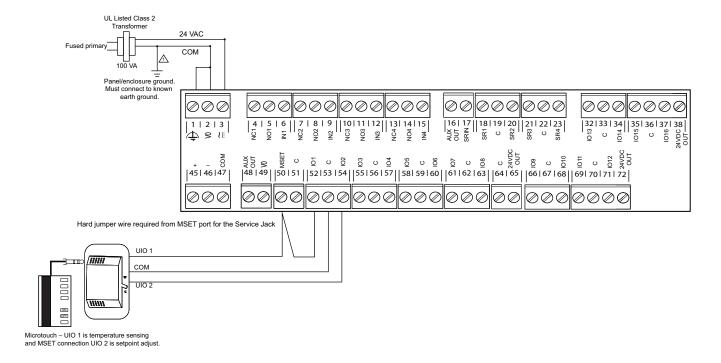
Fig. 26 Alerton Unitary Controller wiring with Microtouch (Large Variant)
