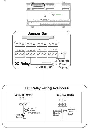
Fig. 21 SPDT Relay Wiring Examples
