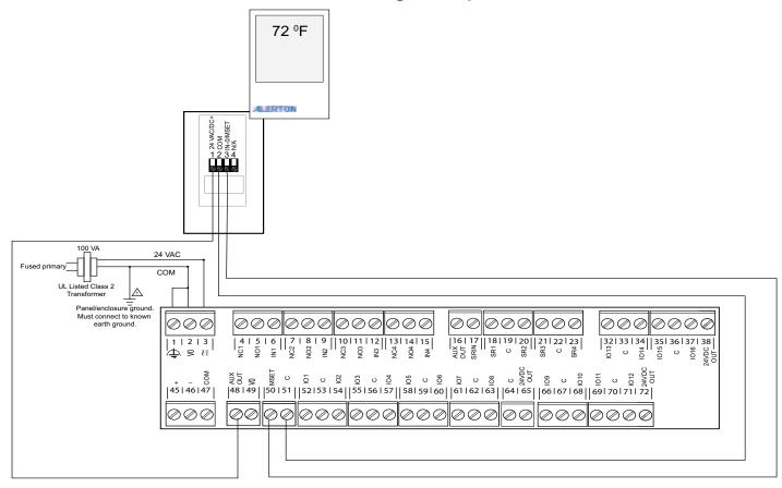
Fig. 22 Alerton Unitary Controller wiring with Microset 4 (Large Variant)
