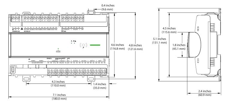
Fig. 3 Alerton Unitary Controller (Small Housing) Dimensions
