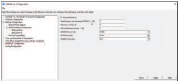
Fig. 39 Modbus Configuration
