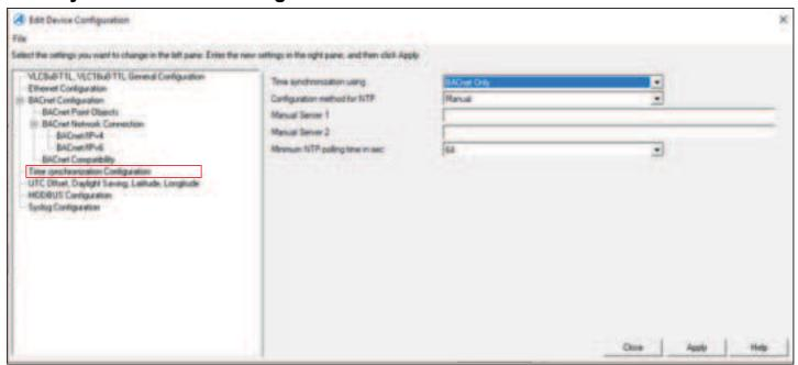
Fig. 37 Time Synchronization Configuration
