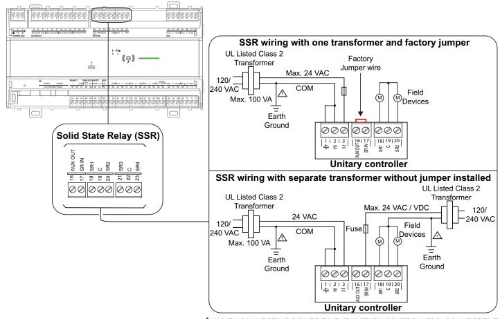
⚠ WHEN CONNECTING POWER TO THE UNITARY CONTROLLERS, CONNECT THE COM OF THE VAC SECONDARY CIRCUIT TO A KNOWN EARTH GROUND.
