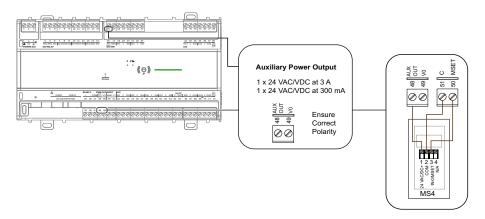
Fig. 20 Auxiliary Wiring Examples
