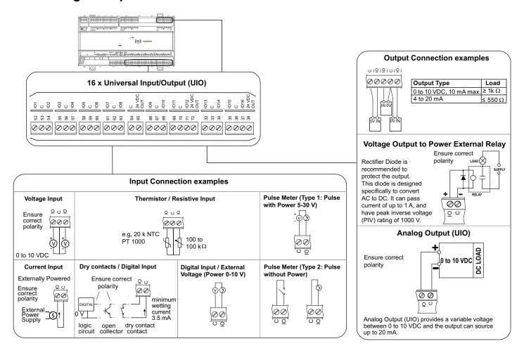
Fig. 18 Universal IO Wiring Examples
