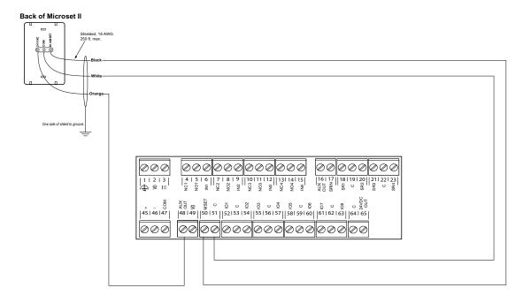
Fig. 25 Alerton Unitary Controller wiring with Microset II (Small Variant)
