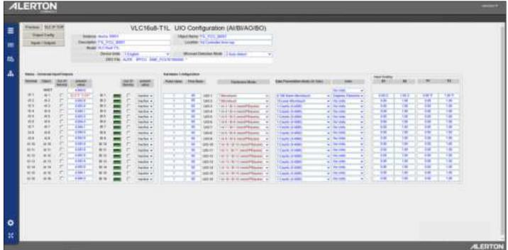
Fig. 56 Unitary Hardware Mode I/O Configuration (Inputs)
