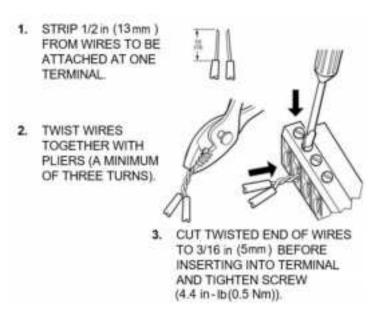
Fig. 10 Attaching Two or More Wires at Terminal Block
