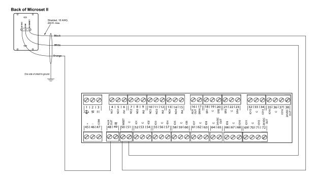
Fig. 24 Alerton Unitary Controller wiring with Microset II (Large Variant)
