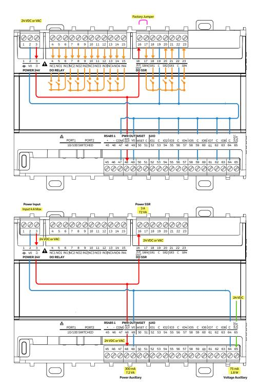
Fig. 12 Internal Wiring Small controller
