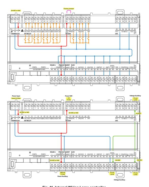
Fig. 11 Internal Wiring Large controller
