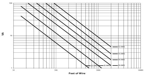
Fig. 8 Determining the appropriate wire size
