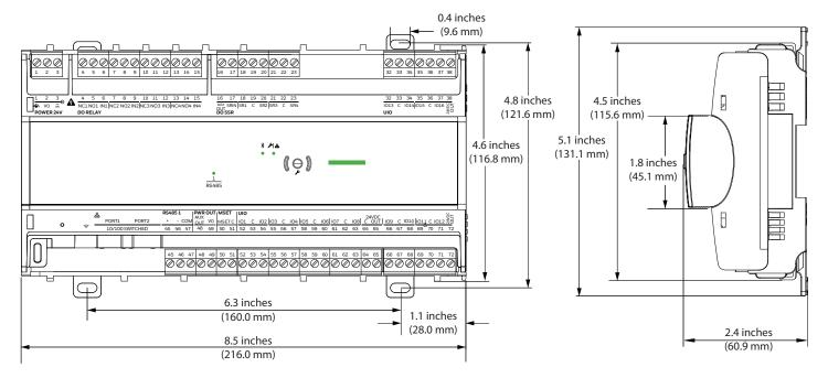
Fig. 2 Alerton Unitary Controller (Large Housing) Dimensions
