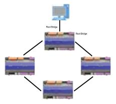
Fig. 74 Root Bridge Example 1
