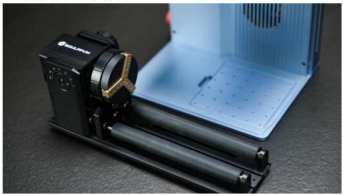
2. Place the materials on the rotary roller and put the roller accessory on the machine working platform.
